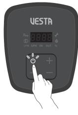
When the water heater is on, the water temperature which has been set recently will appear on the digital display.
